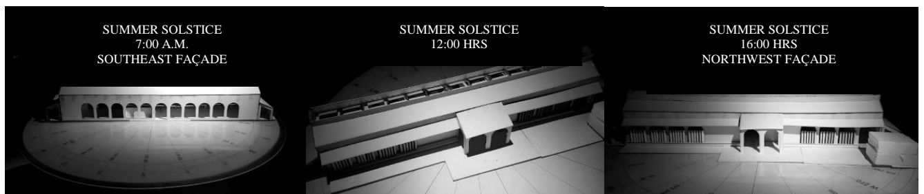
Figure 9. Solar control devices on summer solstice 7:00, 12:00 and 16:00 hrs. Photographs by Tania Osorio using the heliodon
